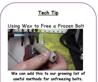
useful methods for unfreezing bolts. Here, you heat the frozen nut with a torch and then melt candle wax into the bolt threads. Repeat as needed until the nut can be worked free.
