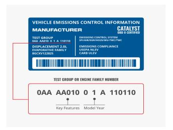
All OBD applications in the <u>WALKER® CALCAT® CARB-COMPLIANT CATALOG</u> reference an EFN. Be sure to verify your EFN to avoid misapplication of the replacement catalytic converter. If the label is missing, it is necessary to contact the OE dealer for the information, or to order a new Emission Control Information Label.
